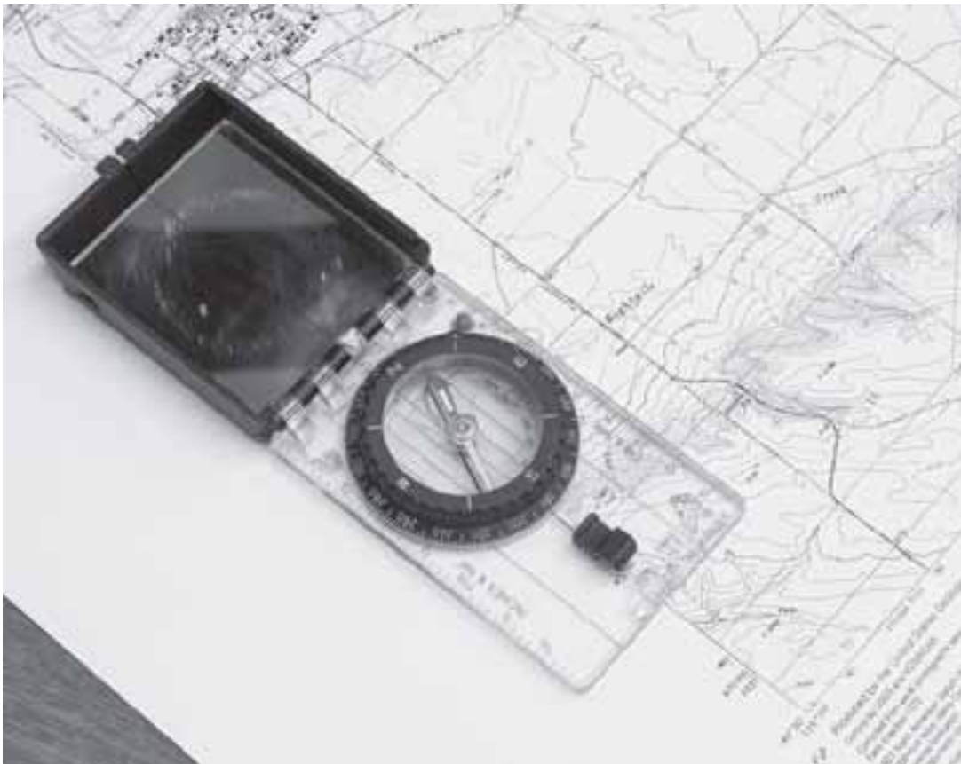
Figure 6-2. Orienting a map with compass.
