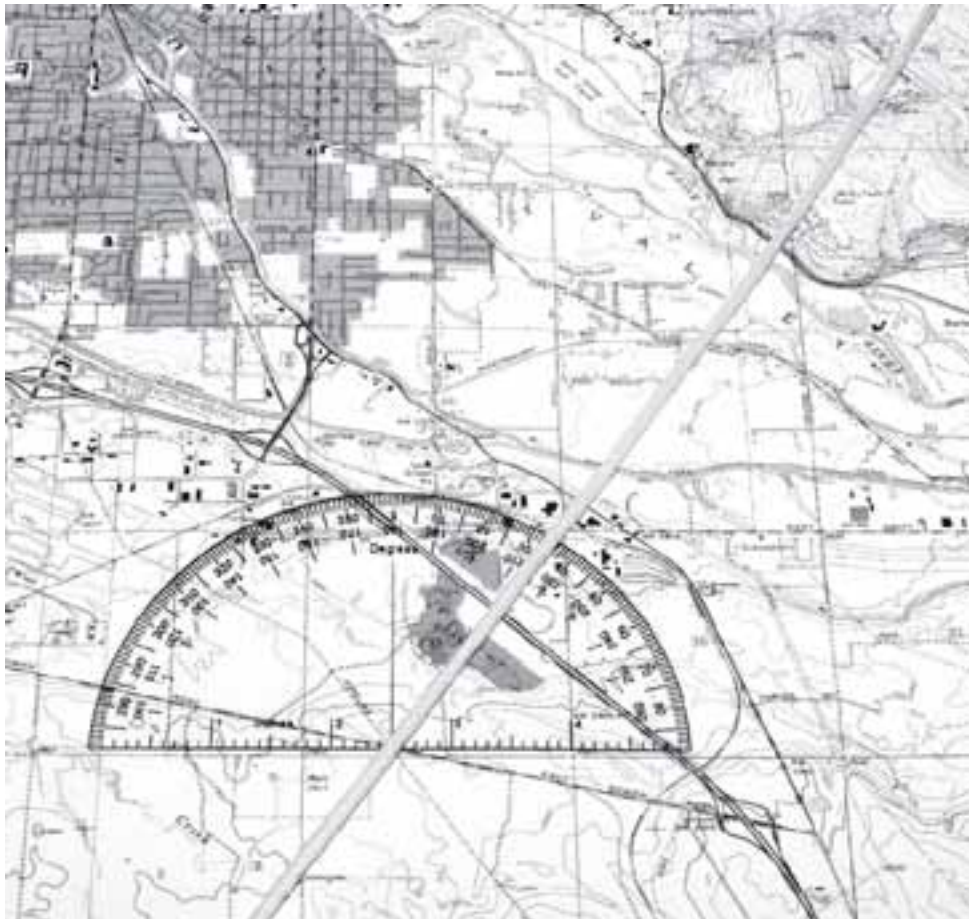
Figure 6-3. Measuring a bearing with a protractor.
