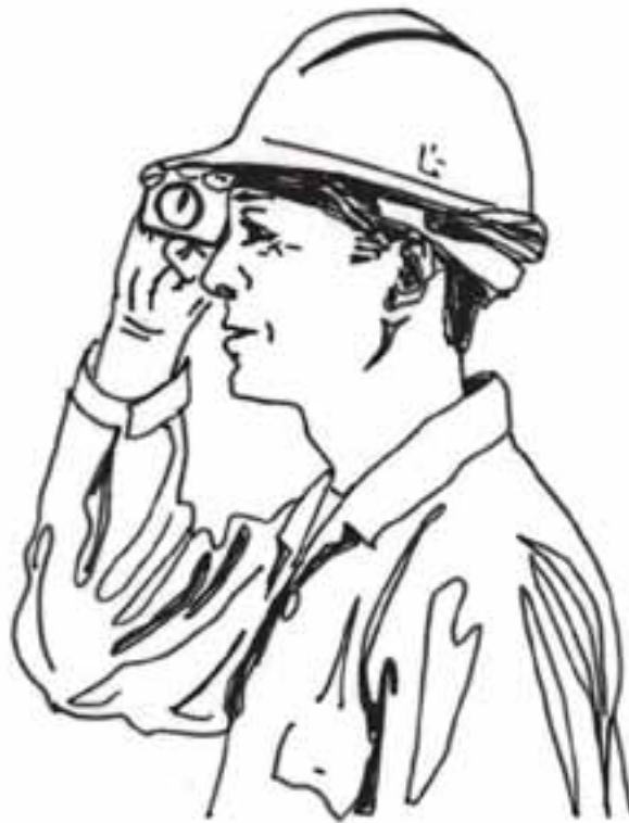
Figure 4-8. Estimating slope with a clinometer.
